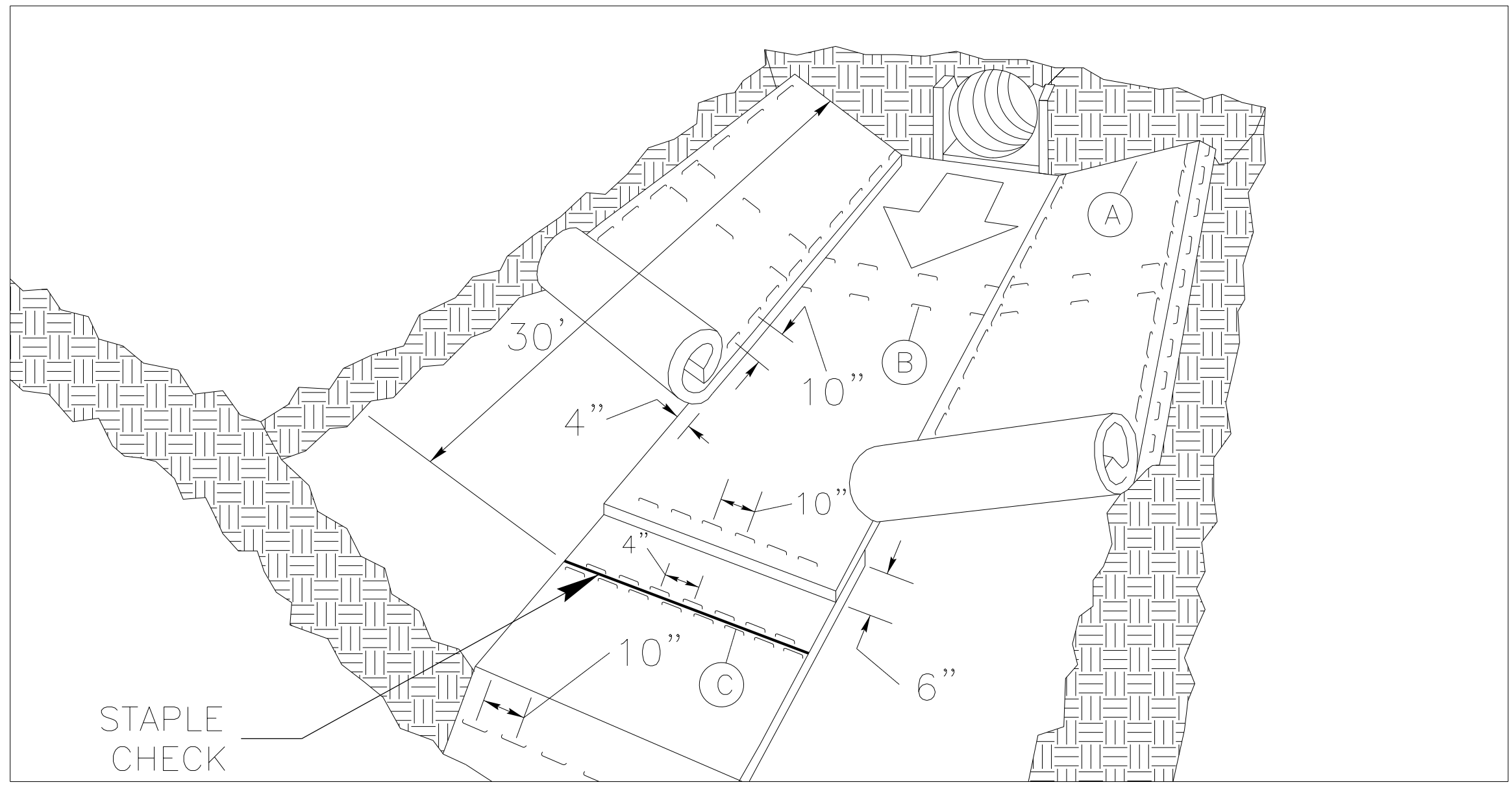
MATTING IN DITCHES
